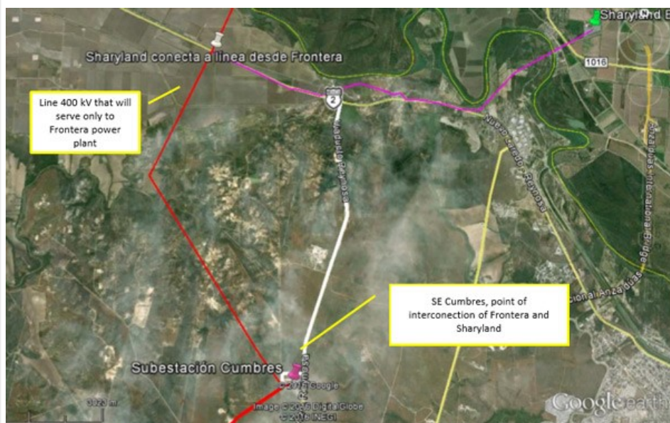
ERCOT Frontera tie to Mexico | Fistera Energy
